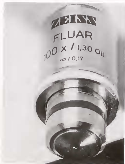
Figure 1. An objective lens with typical markings. Although this is a Zeiss lens, most manufacturers use similar markings.
